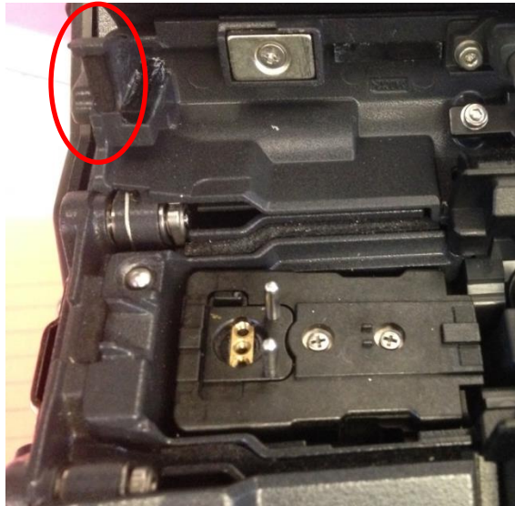
Figure 4: Left side of splicer with foam pad on clamshell lid.
